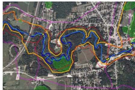
Figure 1: Reach number T02.02 depicting wetlands in green, main stem of the river in royal blue, thalweg in dotted cyan blue, subwatersheds in pink, river corridor in red, valley walls in orange, reach points as yellow dots and bridges as yellow squares.
