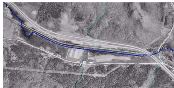
Figure 4: Channel straightening on the Castleton River, reach T02.13. This reach also shows modifications to the floodplain, including roads, rail and some development.
